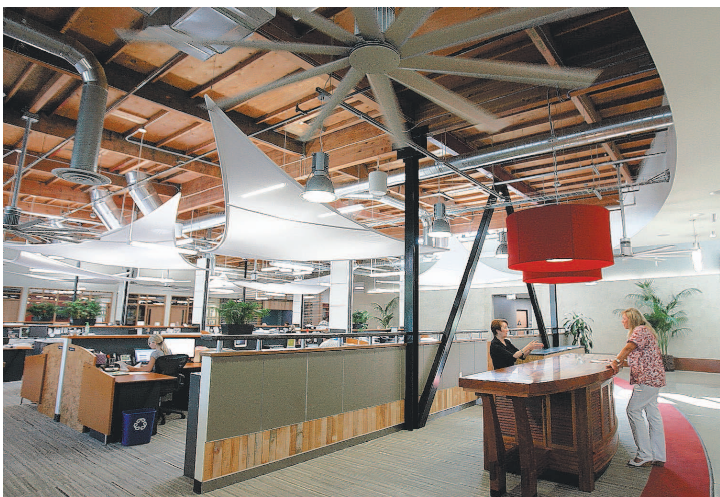
Construction company DPR took a drab industrial space and made it green by installing operable windows, fans, photovoltaic cells and sustainable materials, and reconfiguring a typical office space into an open office plan. JOHN GASTALDO • U-T
